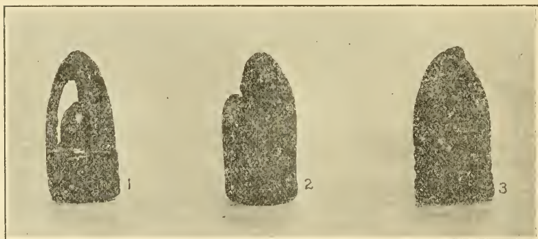
Fig. 1. Explosive bullet, never fired from gun, with outer lead jacket cut away, exposing the copper shell containing the high explosive.
